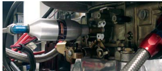
Meth nozzle spraying directly through a modified carb offers perfect distribution and atomization
