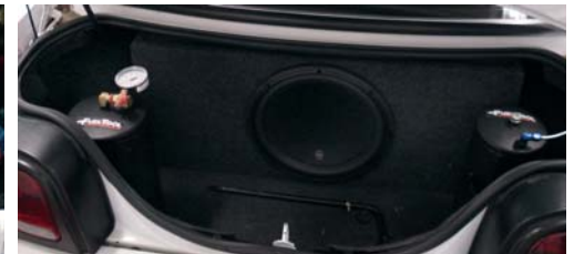
Another mounting option as installed in the trunk of a Mustang where the tanks are split
