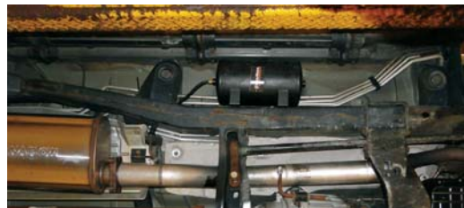
Air tank mounted in a Dodge Durango under the passenger side keeping the tanks hidden
