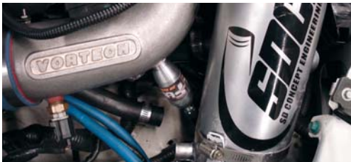
Meth nozzle as installed on a '97 Cobra
