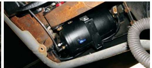
The meth tank mounted in the back quarter panel of a Durango doesn't take up any interior room of the vehicle
